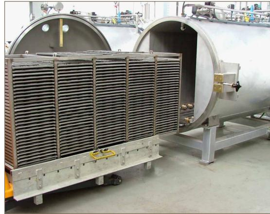
Fig. 3 Rack with green parts loaded on trays, ready to be inserted into LÖMI debinding plant EBA-2500
