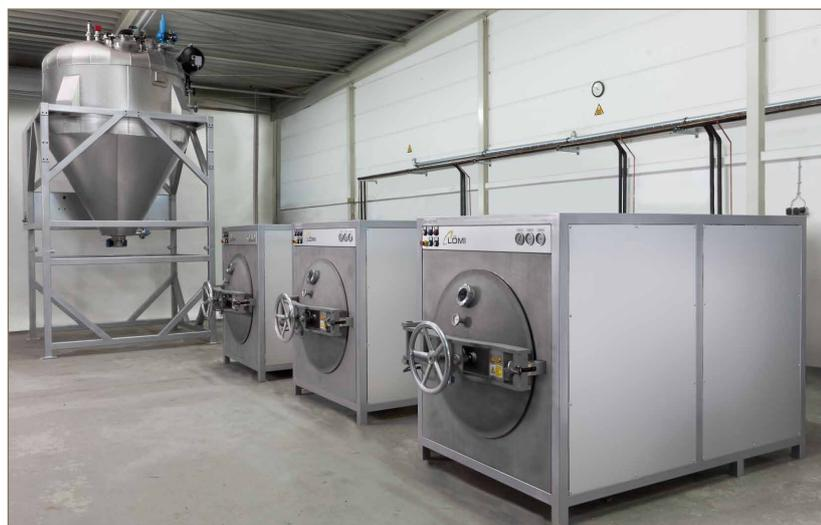
Fig. 4 Three debinding furnaces EBA-900 with a parallelly operated solvent recovery system VDA-3000, shortly before commissioning at a major Indian customer
