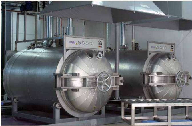
Fig. 2 LÖMI debinding plants EBA-2500 for the high volume debinding of powder injection moulded parts
